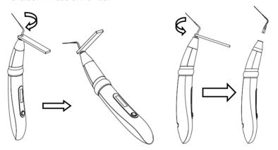
Tighten clockwise to install the tip
